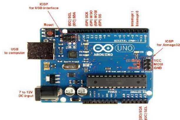
Figure 3: Arduino UNO Based on ATMega-328 Microcontroller
