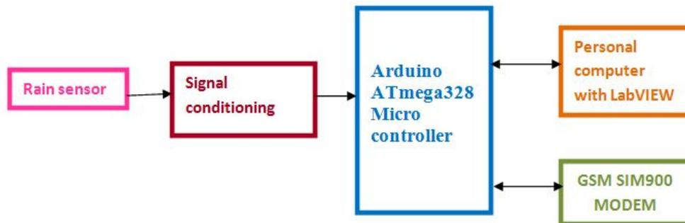
**Figure 1: Block Diagram of Rain Fall Detector with Arduino**
